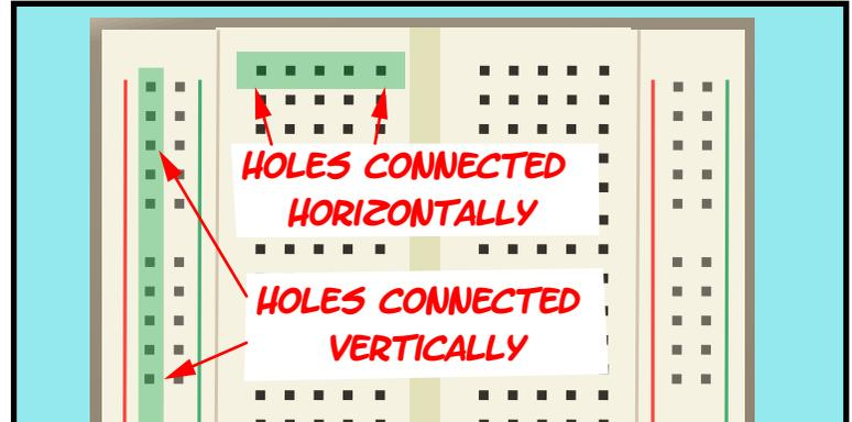
THIS BREADBOARD HAS 2 ROWS OF HOLES RUNNING DOWN THE LEFT AND RIGHT SIDE, AND 5 ROWS OF HOLES ON EITHER SIDE OF A MIDDLE INDENTATION. THE SIDE ROWS ARE CONNECTED **VERTICALLY**, EACH ROW OF 5 HOLES IN THE MIDDLE ARE CONNECTED **HORIZONTALLY**.
