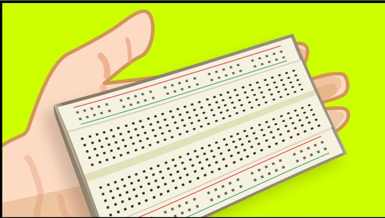
HOW DO WE CONTROL OBJECTS THAT ARE NOT ON THE ARDUINO BOARD? WE WILL CONNECT THE ARDUINO TO A **SOLDERLESS BREADBOARD**. THIS WILL ALLOW US TO QUICKLY SET UP AND TEST CIRCUITS.
