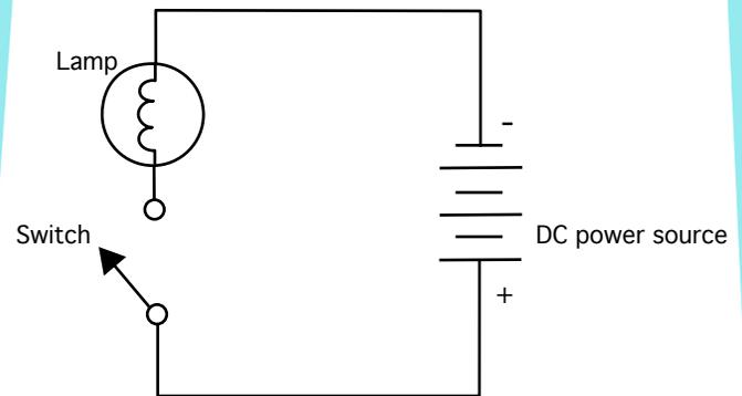
THIS IS A **SCHEMATIC** OF THE SAME CIRCUIT (IT REPRESENTS THE CIRCUIT USING SYMBOLS FOR THE ELECTRONIC COMPONENTS). WHEN THE SWITCH IS CLOSED, CURRENT FLOWS FROM THE POWER SOURCE AND LIGHTS THE LAMP.
