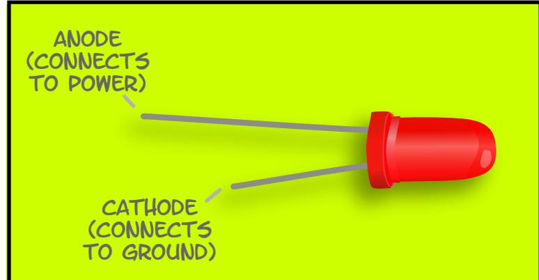
WHEN CURRENT FLOWS THROUGH A **LED (LIGHT EMITTING DIODE)** IN THE RIGHT DIRECTION, IT LIGHTS UP. WE'LL ATTACH AN LED TO THE BREADBOARD, THEN TO THE ARDUINO SO WE CAN CONTROL IT WITH CODE.
