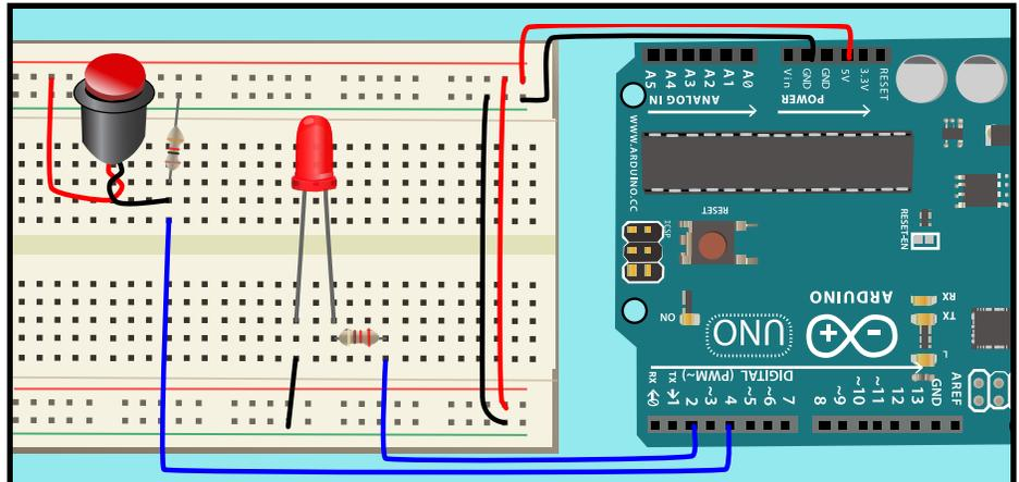
CONNECT ONE END OF A MOMENTARY SWITCH TO PIN 4 ON THE ARDUINO, WITH A 10K RESISTOR CONNECTED TO GROUND ATTACHED TO THE SAME END. ATTACH THE OTHER END TO POWER. WE WILL LEAVE THE LED ATTACHED TO THE SAME PIN.
