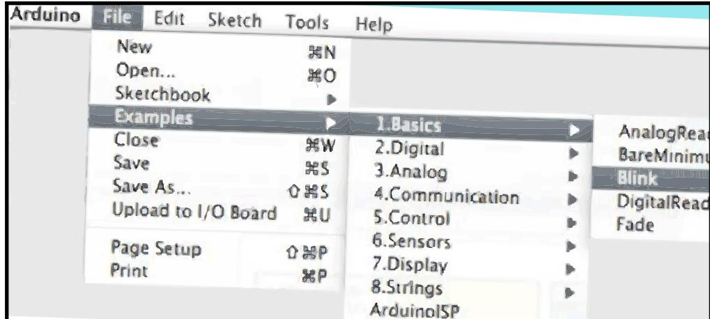
THE ARDUINO IDE ALLOWS YOU TO WRITE **SKETCHES**, OR **PROGRAMS** AND UPLOAD THEM TO THE ARDUINO BOARD. OPEN THE **BLINK** EXAMPLE IN THE FILE MENU. FILE > EXAMPLES > 1.BASICS > BLINK.
