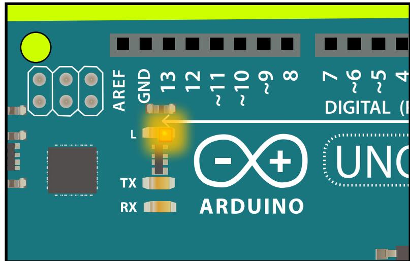
THE LED AT PIN 13 ON THE ARDUINO STARTS BLINKING.
