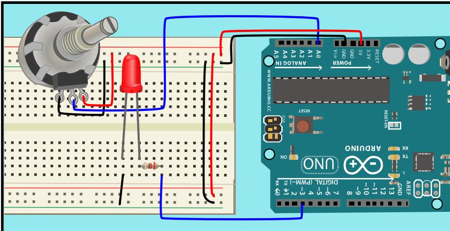
LET'S USE THE CHANGING VALUES WE RECEIVE FROM THE POT AS A DIMMER TO LIGHT AN LED. PUT THE LED BACK INTO THE BOARD, ATTACHED TO THE ARDUINO AT PIN 3.
