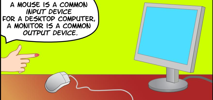
MICROCONTROLLERS USE **INPUTS** AND **OUTPUTS** LIKE ANY COMPUTER. INPUTS CAPTURE INFORMATION FROM THE USER OR THE ENVIRONMENT WHILE OUTPUTS DO SOMETHING WITH THE INFORMATION THAT HAS BEEN CAPTURED.
