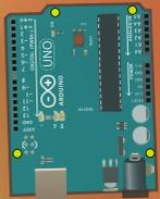
ATTACHING THE ARDUINO TO A COMPUTER WITH A USB CABLE WILL SUPPLY THE 5 VOLTS OF POWER WE NEED AND ALLOW US TO START PROGRAMMING.
