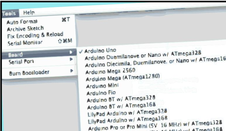
LAUNCH THE ARDUINO SOFTWARE. IN THE TOOLS MENU, SELECT THE BOARD YOU ARE USING (TOOLS > BOARD). FOR EXAMPLE, ARDUINO UNO.
