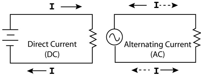
THERE ARE TWO COMMON TYPES OF CIRCUITS, **DIRECT CURRENT** AND **ALTERNATING CURRENT**. IN A DC CIRCUIT, THE CURRENT ALWAYS FLOWS IN ONE DIRECTION. IN AC, THE CURRENT FLOWS IN OPPOSITE DIRECTIONS IN REGULAR CYCLES. WE WILL ONLY TALK ABOUT DC CIRCUITS HERE.
