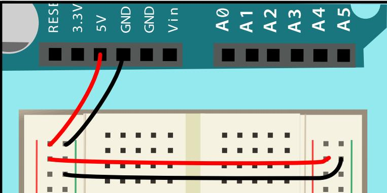
WE WILL CONNECT **POWER** AND **GROUND** FROM THE ARDUINO BOARD TO THE VERTICALLY CONNECTED STRIPS ON THE LEFT AND RIGHT WITH 22 GAUGE WIRE. OTHER COMPONENTS CAN BE ATTACHED TO THE HOLES IN THE MIDDLE AND TO POWER AND GROUND AS NEEDED.
