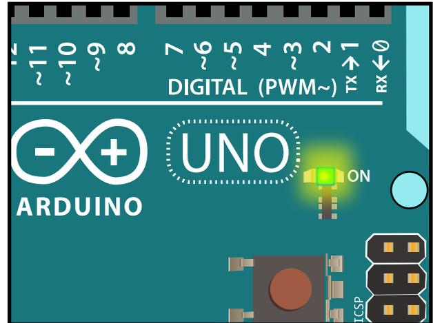
WHEN YOU HAVE INSTALLED THE SOFTWARE, CONNECT THE ARDUINO. AN LED MARKED ON SHOULD LIGHT UP ON THE BOARD.
