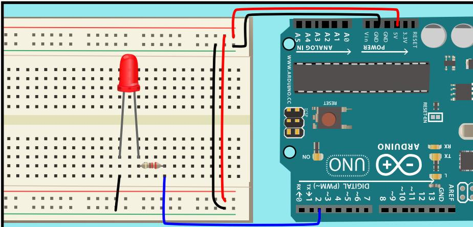
THE ANODE IS CONNECTED TO PIN 2 ON THE ARDUINO THROUGH A 220 OHM RESISTOR. THE CATHODE IS CONNECTED TO GROUND. PINS 2 THROUGH 13 CAN BE CONFIGURED AS DIGITAL INPUTS OR OUTPUTS. CLICK **NEW** BUTTON TO START A SKETCH.
