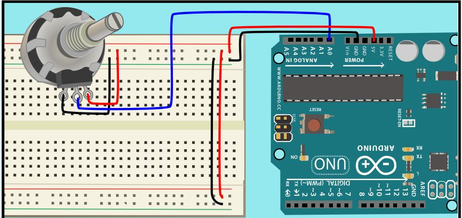
ATTACH THE MIDDLE PIN ON THE POTENTIOMETER TO ANALOG PIN A0. ATTACH ONE END OF THE POT TO POWER, THE OTHER TO GROUND.
