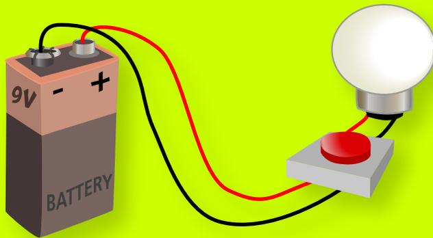
NOW LET'S LOOK AT A SIMPLE **CIRCUIT**. EVERY CIRCUIT IS A CLOSED LOOP THAT HAS AN **ENERGY SOURCE** (BATTERY) AND A **LOAD** (LAMP). THE LOAD CONVERTS THE ELECTRICAL ENERGY OF THE BATTERY AND USES IT UP. THIS ONE HAS A SWITCH TOO.
