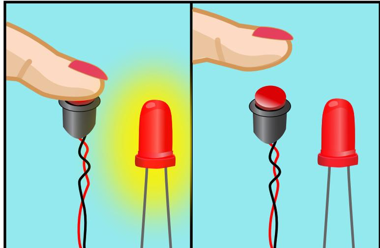
THE LED LIGHTS WHEN THE SWITCH IS HELD DOWN.
