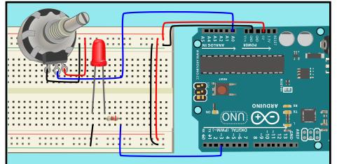
LET'S USE THE CHANGING VALUES WE RECEIVE FROM THE POT AS A DIMMER TO LIGHT AN LED. PUT THE LED BACK INTO THE BOARD, ATTACHED TO THE ARDUINO AT PIN 3.
