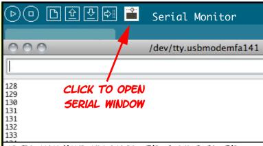
AFTER YOU HAVE UPLOADED THE SCRIPT TO THE ARDUINO, CLICK THE SERIAL MONITOR BUTTON IN ORDER TO SEE THE VALUES AS YOU TURN THE POT. A WINDOW WILL OPEN, AND YOU WILL SEE VALUES RANGING FROM 0 TO 1024 AS THE POT IS TURNED.
