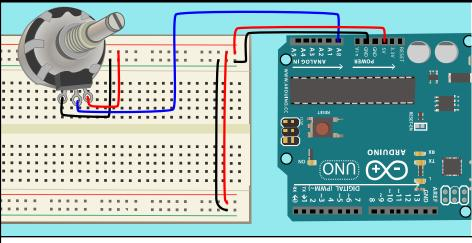
ATTACH THE MIDDLE PIN ON THE POTENTIOMETER TO ANALOG PIN AO. ATTACH ONE END OF THE POT TO POWER, THE OTHER TO GROUND.
