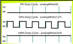
WE'LL USE PULSE WIDTH MODULATION (PWM). THIS IS A METHOD OF SIMULATING AN ANALOG VALUE BY MANIPULATING THE VOLTAGE, TURNING IT ON AND OFF AT DIFFERENT RATES, OR DUTY CYCLES. YOU CAN USE PWM WITH PINS 3, 5, 6, 9, 10, AND 11.
