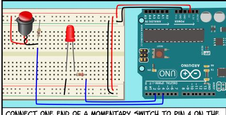
CONNECT ONE END OF A MOMENTARY SWITCH TO PIN 4 ON THE ARDUINO, WITH A 10K RESISTOR CONNECTED TO GROUND ATTACHED TO THE SAME END. ATTACH THE OTHER END TO POWER. WE WILL LEAVE THE LED ATTACHED TO THE SAME PIN.
